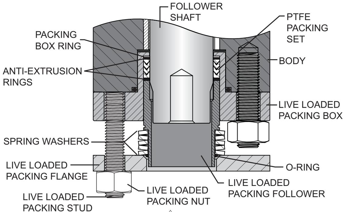
Figure 7 Live Loaded Packing Configuration - Outboard
