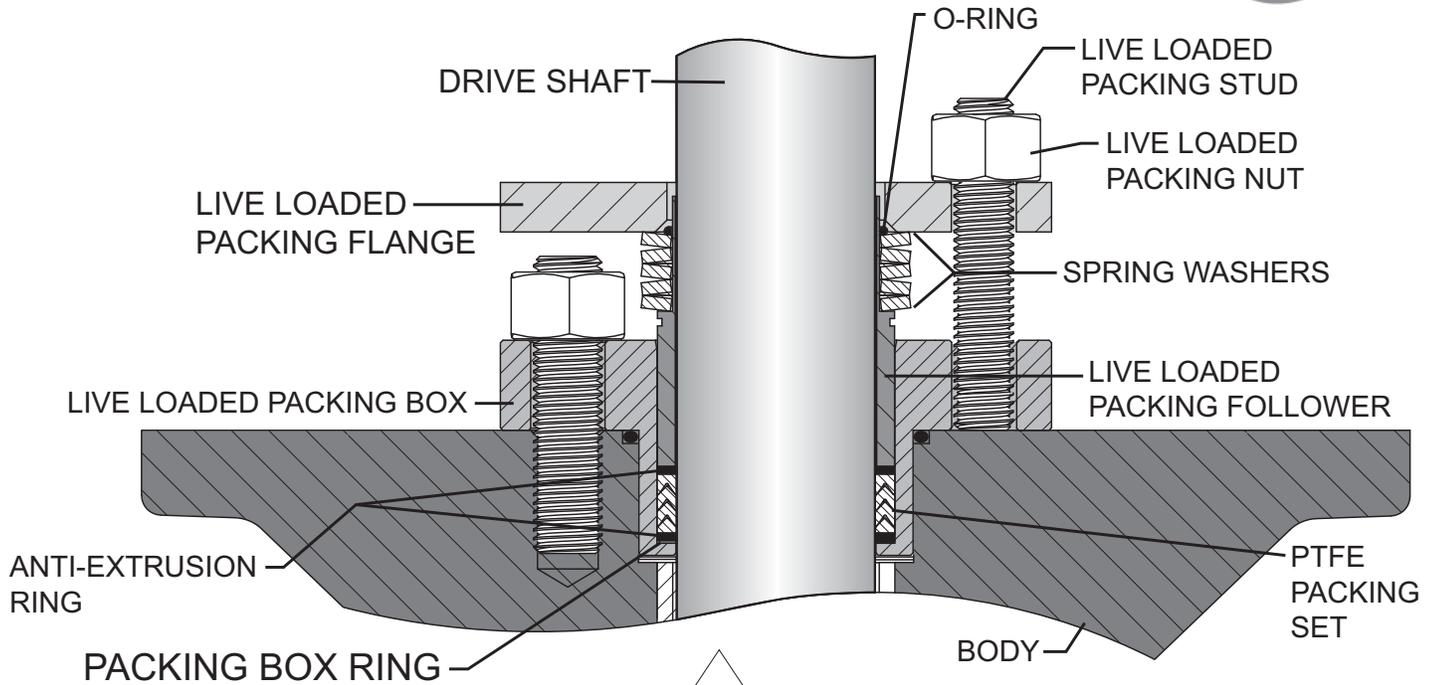
Figure 6 Live Loaded Packing Configuration - Inboard
