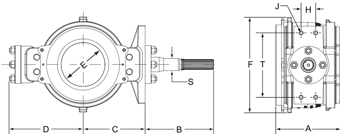
Figure 2 Model 590 Valve Dimensions Diagram
