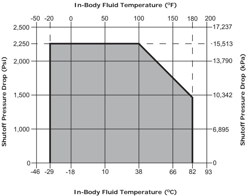
NOTE: Do not exceed the pressure/temperature limitations in the above chart or the body rating, whichever is lower.
