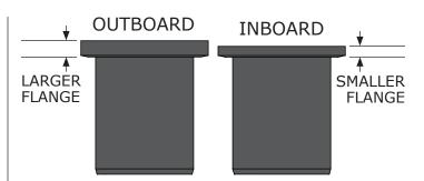
DIFFERENTIATION BETWEEN THE INBOARD AND OUTBOARD BEARINGS (KEY 3) CAN BE PERFORMED THROUGH VISUAL INSPECTION. THE INBOARD BEARING HAS A SMALLER FLANGE COMPARED TO THE OUTBOARD BEARING. THIS SMALLER FLANGE ALLOWS FOR THE ACCOMMODATION OF THE THRUST WASHER (KEY 7) BETWEEN THE BEARING AND THE BALL (KEY 6).
