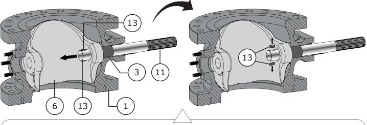
Figure 26 16 Inch Drive Shaft Pin Removal
