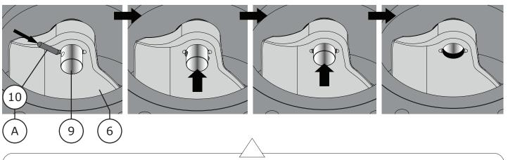
Figure 53 16 Inch Follower Shaft Pin Installation
