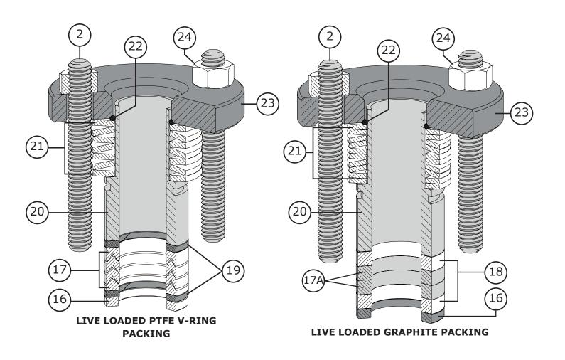
Figure 60 Packing Configuration Diagrams (Refer to Figure 61 & 62 for Spring Washer, Key 21, Arrangements)
