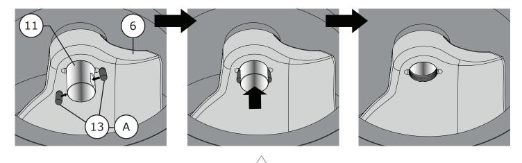
Figure 52 16 Inch Drive Shaft Pins Installation
