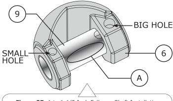
**Figure 37** 1 to 1-1/2 Inch Follower Shaft Installation
