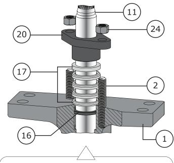
Figure 8 Standard Packing Removal
