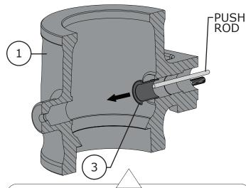
Figure 29C 3 to 16 Inch Inboard Bearing Removal
