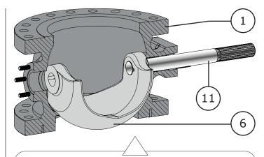
Figure 50 16 Inch Drive Shaft / Ball Installation Step 2
