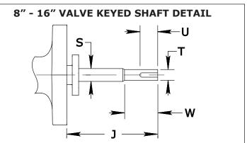
Figure 2 Typical Valve Assembly Diagram and Dimensions
