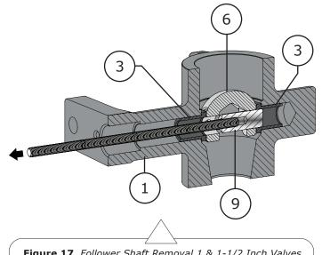
Figure 17 Follower Shaft Removal 1 & 1-1/2 Inch Valves
