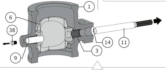
Figure 19 3 to 12 Inch Drive Shaft / Pipe Plug Removal
