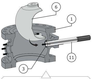
Figure 49 16 Inch Drive Shaft / Ball Installation Step 2
