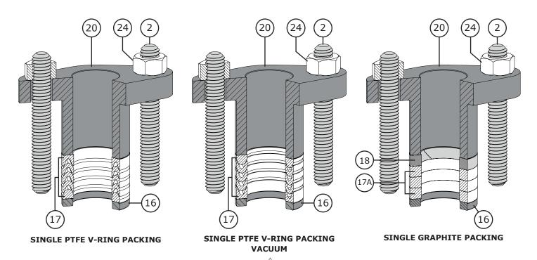
Figure 59 Standard Packing Configuration Diagrams
