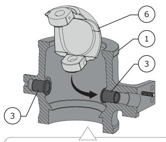
Figure 44 2 to 12 Inch Valve Ball Installation
