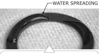
Figure 31 Bondable Side - Thrust Washer Water Test
