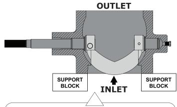
Figure 14 Valve Placement for 6" to 16" Disassembly
