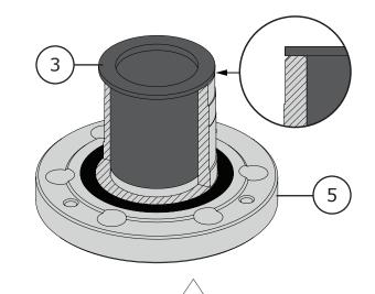
Figure 36 16 Inch Outboard Bearing Installation
