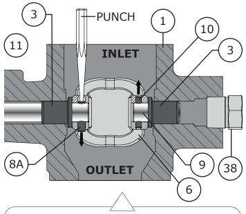
Figure 15 2 Inch Valve Pin Removal
