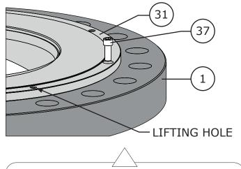
Figure 65 Seal Protector Ring Retaining Parts Installation
