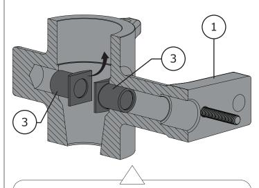
Figure 28 Old Style 1 & 1-1/2 Inch Outboard Bearing Removal
