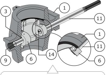
Figure 47 3 to 12 Inch Valve Drive Shaft Installation
