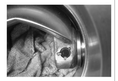
Figure 41 1 to 2 Inch Shaft Connection Stake Example
