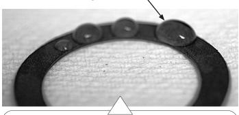
Figure 30 Bearing Side - Thrust Washer Water Test
