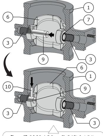
Figure 45 6 & 8 Inch Follower Shaft / Pin Installation
