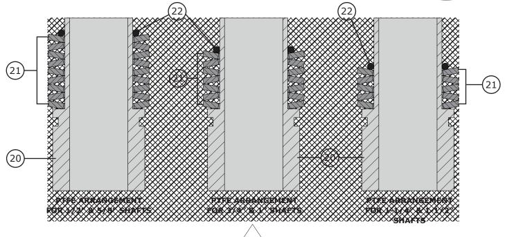
Figure 61 Live Loaded PTFE Spring Washer (Key 21) Arrangements
