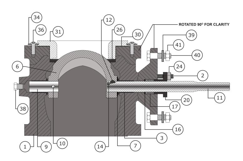
\*NOTE: 3 AND 4 INCH VALVES DO NOT HAVE A THRUST WASHER (KEY 7).
