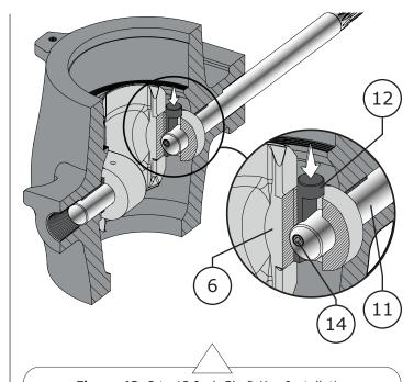
Figure 48 3 to 12 Inch Shaft Key Installation
