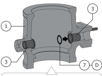
Figure 42 Thrust Washer Installation
