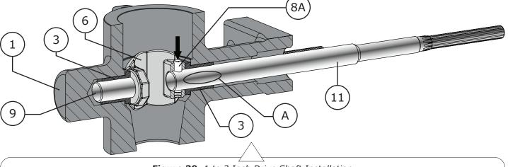
Figure 39 1 to 2 Inch Drive Shaft Installation
