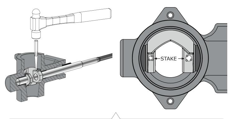
Figure 40 1 to 2 Inch Shaft Connection Pin Stake Locations (2 inch valve stake locations are 180° apart)
