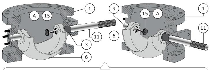
Figure 54 16 Inch Shaft Retainer Installation
