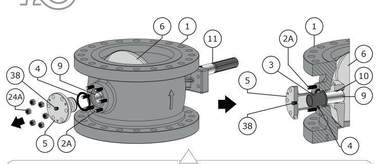
Figure 22 16 Inch Flange / Spiral Wound Gasket / Bearing Removal
